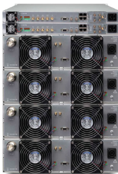
Transmissor DTT 2,0kW Single-Drive Ultra-Wideband Doherty em 14 HU
